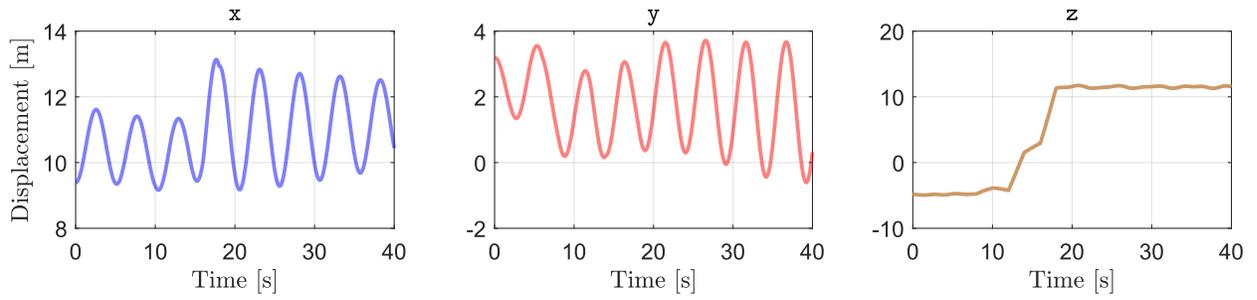
**FIGURE 4: UNSHAPED RESPONSE OF THE ROBS TIP.**
