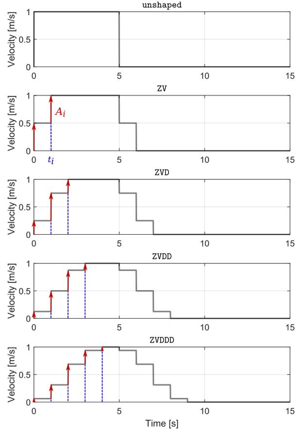
FIGURE 2: INPUT SHAPING CONVOLUTION PROCESS.
