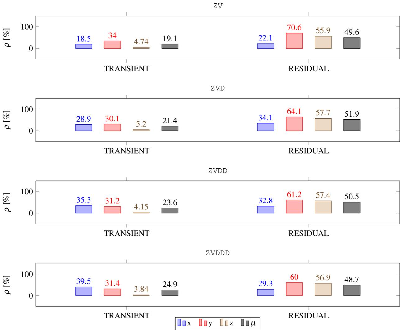
**FIGURE 5: VIBRATION SUPPRESSION INDEX FOR THE DIFFERENT SHAPERS.**
