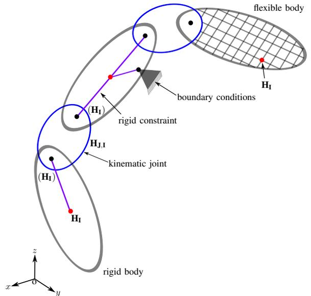
Fig. 1. General description of a robotic manipulator:  $\mathbf{H}_I$  are nodal frames,  $\mathbf{H}_{J,I}$  are relative transformations and  $(\mathbf{H}_I)$  are optional frames, used to specify boundary conditions or kinematic joints.
